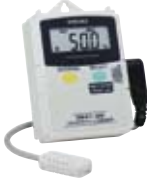
3641-20 -40.0°C to 85.0°C 0.0 to 100.0% rh (using the 9680 sensor)
